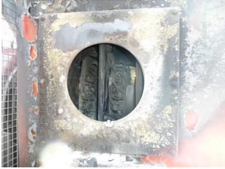
**Figure 1:** *Severe slipring flash over*
