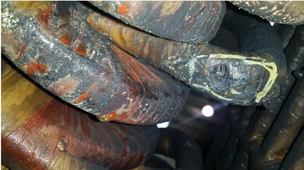
**Figure 3:** *Fault at stator winding series connection*
