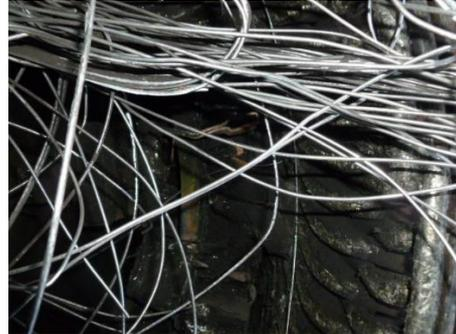
**Figure 2:** *Rotor banding failure*
